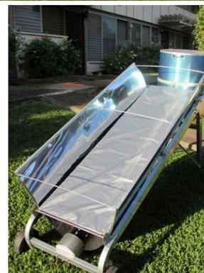
3. The Devos Cooker is another type of solar cooker<sup>31</sup>. This comprises a parabolic concentrator and a table where food can be prepared as well as cooked. This was also trialed by the UNHCR at the Goudoubo Refugee camp but was rejected by the refugees<sup>32</sup>. The reason is not given.
