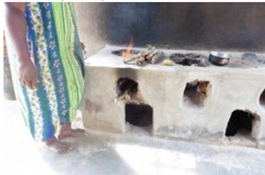
Rocket stoves are also proving popular. These stoves are available in a variety of shapes and sizes but they all have an L-shaped combustion chamber that is insulated. This chamber improves the combustion of the wood and channels the hot gases up to the cooking pot.<sup>4</sup> These means that they are more efficient in cooking the food and use significantly less fuel. Tests have shown that it uses 60% less wood fuel to boil 1L of water and simmer it for 30min.<sup>5</sup>
