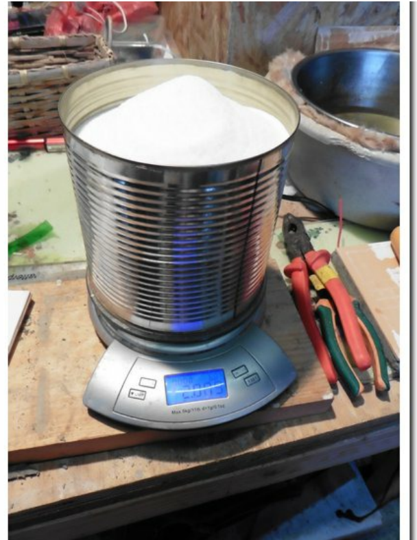
#2 PCM being weighed into PCM vessel
