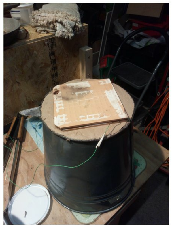
#2 Tile heater trimmed to fit the base of the PCM bucket
