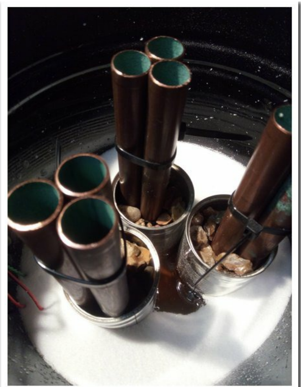
#6 Pillars surrounded by PCM which has just started to melt
