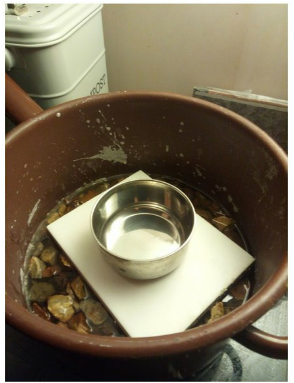
#6 Tile on top of gravel was poor conductor due to minimal contact with gravel
