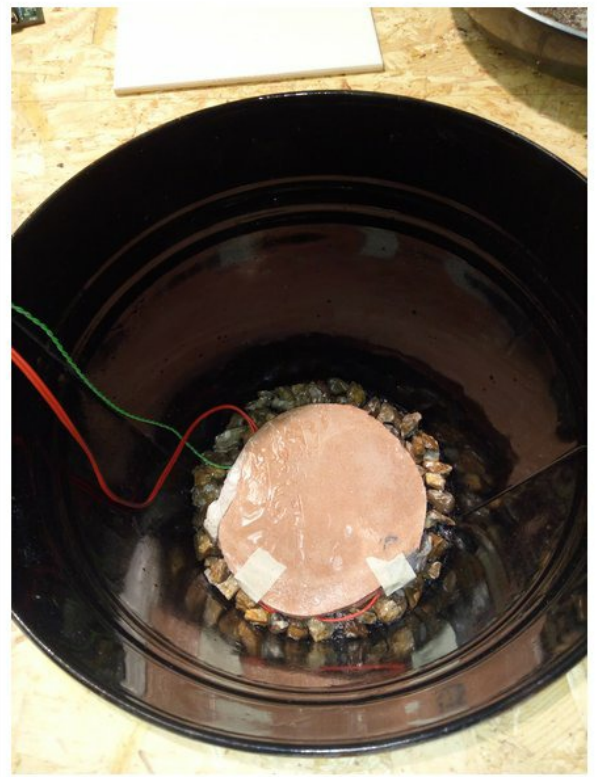
#2 Clay heater tile on top of gravel
