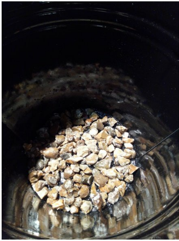
#1 Gravel used as spacer underneath the heater
