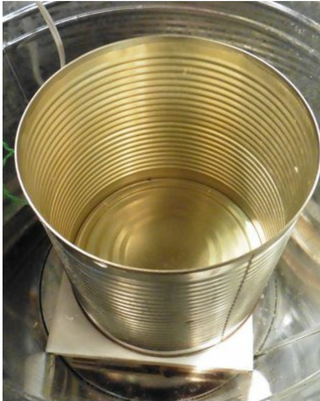
#1 Heater tile on spacers to allow oil circulation. PCM can on top of heater
