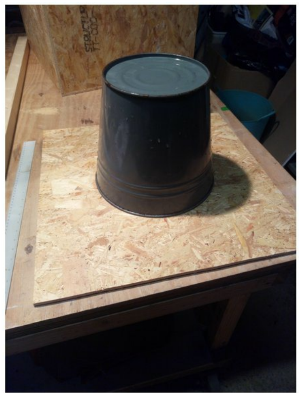
#2 Metal waste bin used as the PCM vessel
