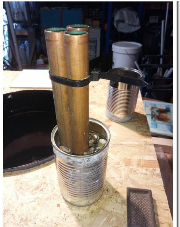
#4 Pipe pillars with gravel filled cant holding the copper pipes in position
