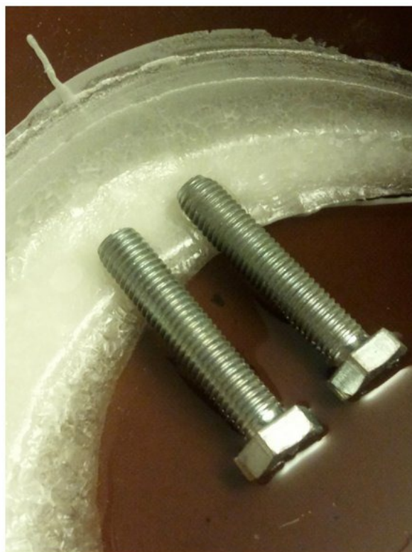
#3 Bolts had minimal impact to surrounding PCM
