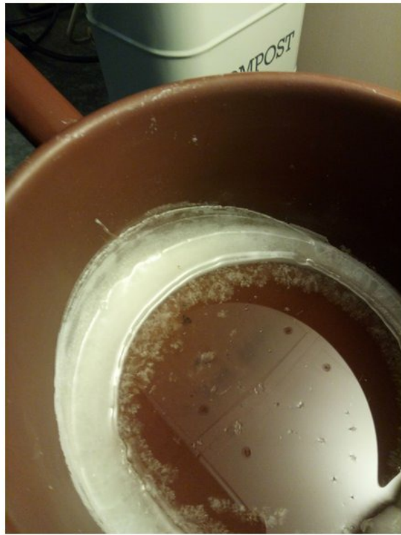
#1 PCM melted in middle but not edges
