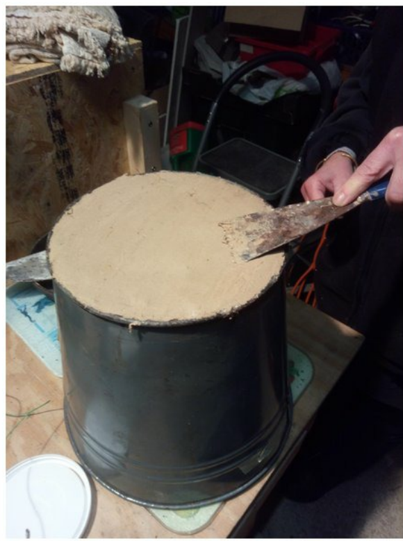
#1 Mortar filling the lipped to prevent an air pocket insulating the PCM bucket
