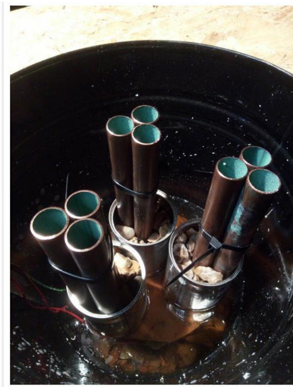
#5 The pillars in position in PCM bucket
