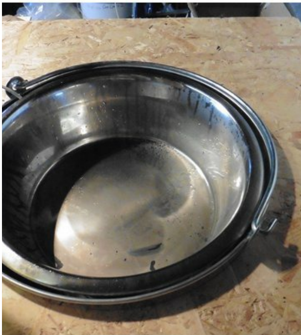
#7 "Dogbow" hotplate resting on PCM vessel within oil bath vessel.
