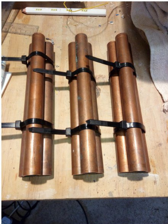
#3 Copper tube pillars held together with cable ties
