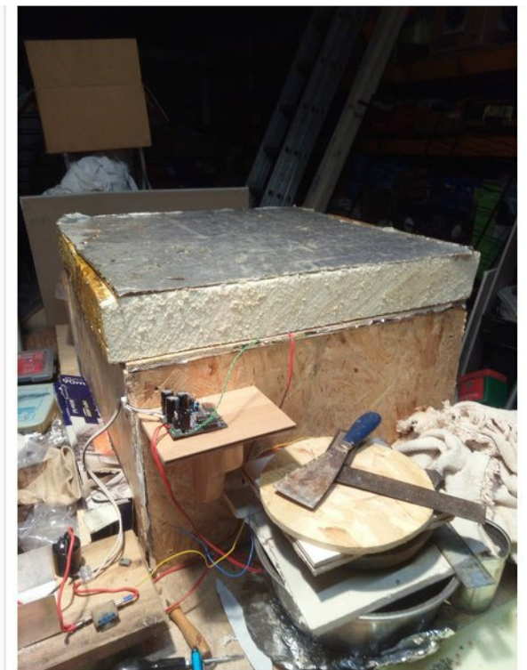
#7 Base assembly under test with temporary insulation on the top
