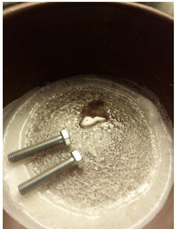
#2 Steel bolts added as heat transfer rods
