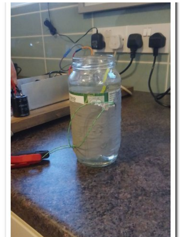
#8 Jar heater under test - note thermometer
