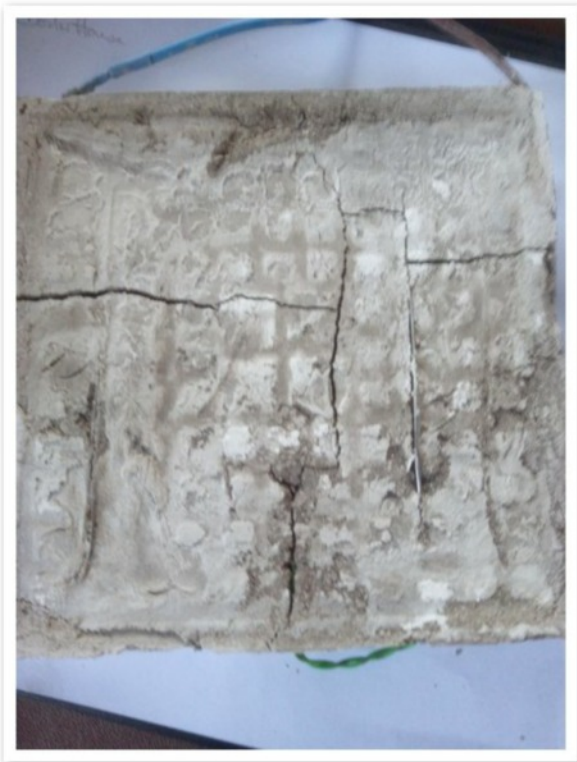
#17 Dried clay shrunk after drying. Tile weak and unserviceable due to exposed wires
