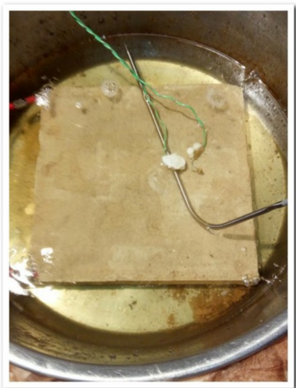
#25 Oil bath being used to condition cement
