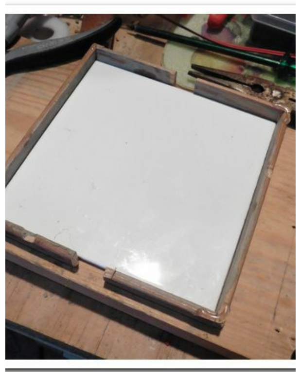
#28 Revised mould to allow wires to protrude in a horizontal plane
