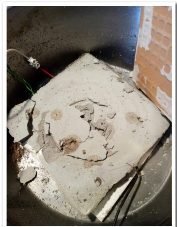
#30 Thermistor connection using a choc block to provide tension support once in cement
