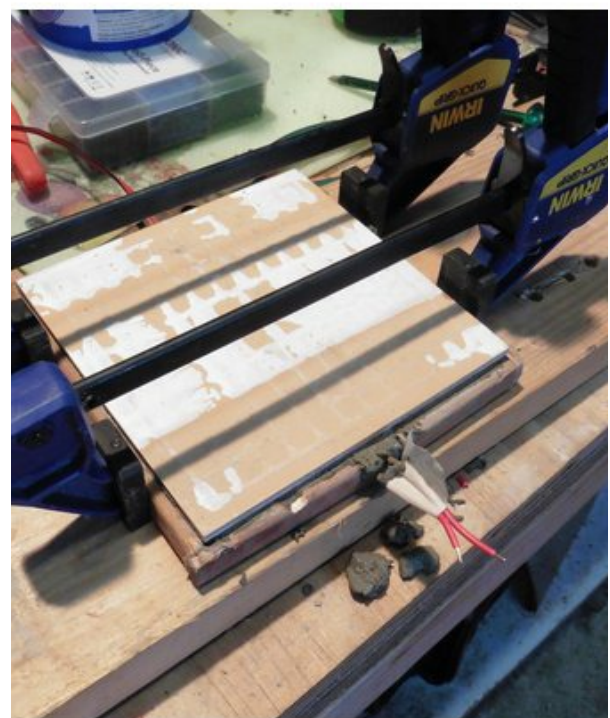
#32 Clamps being used to hold tiles whilst setting
