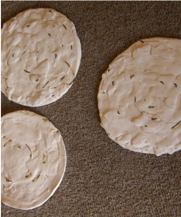
#1 First attempt at clay heaters. Burnt out wire shown as brown flecks
