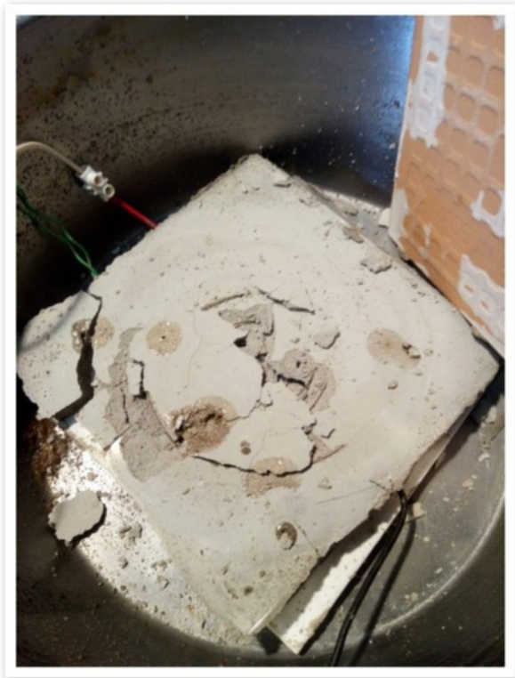
#23 Cement tile blown by heating with retained moisture - A
