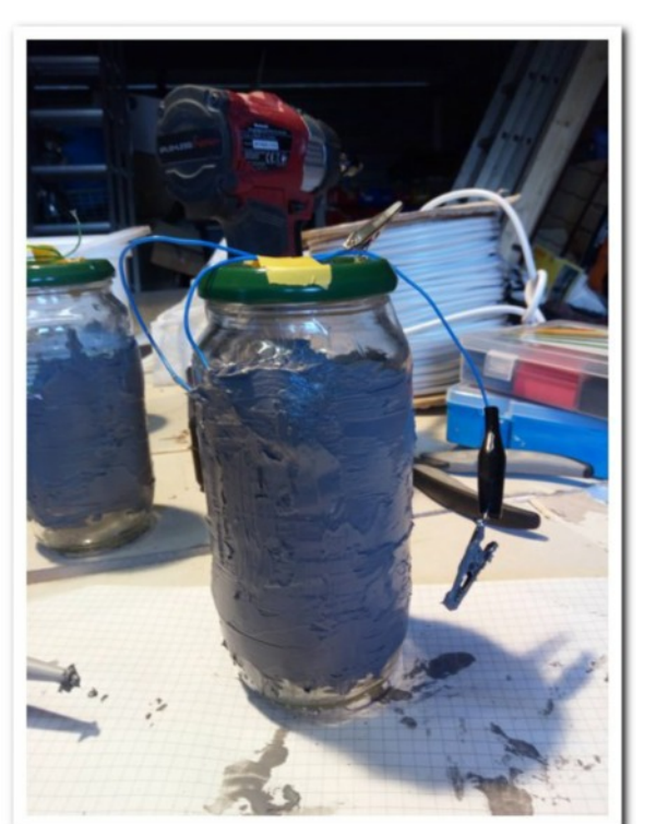
#4 Wire encased with fire cement
