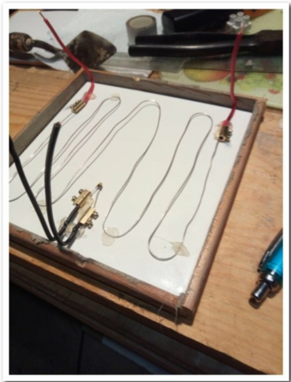
#27 First version of mould showing wires coming out in the vertical plane
