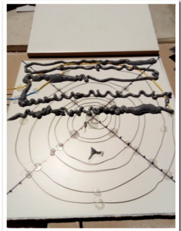
#6 Fabrication - Apply fire cement
