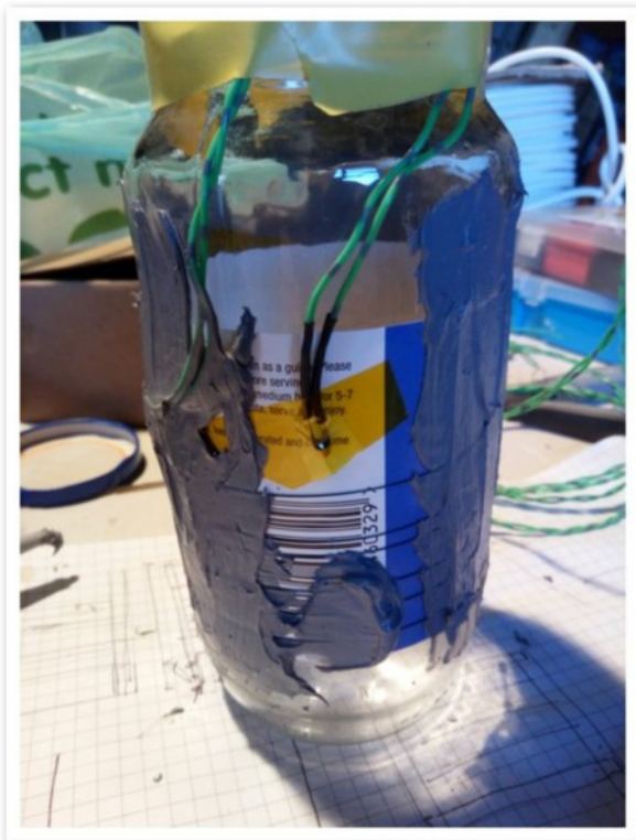
#7 Heat resistant tape holding thermistor
