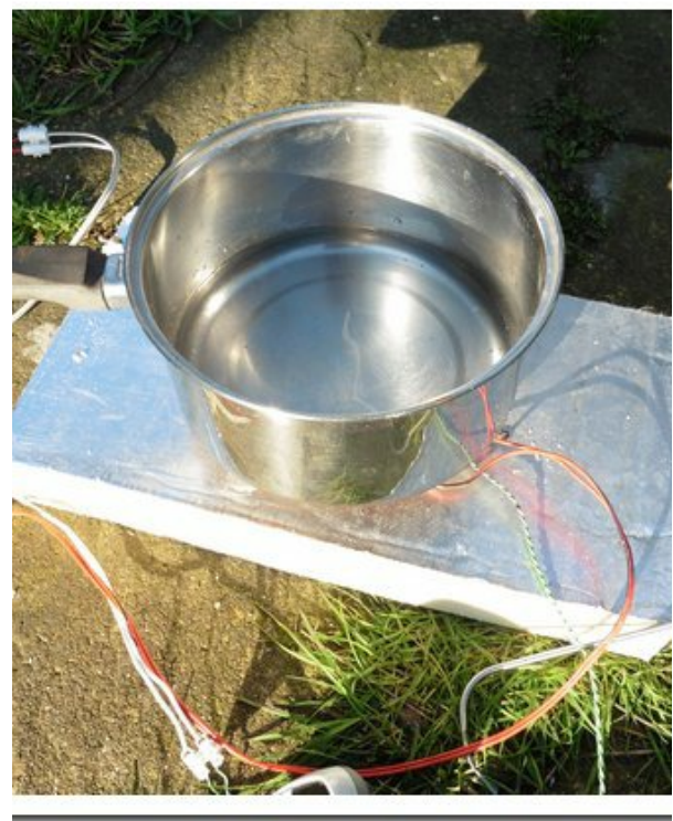
Hotplate trial showing pan on top of clay tile.
