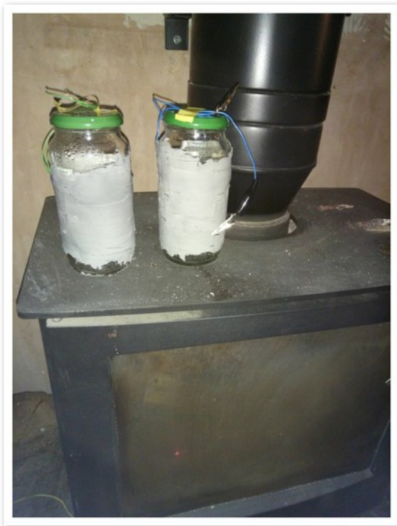
#5 Fire cement being cured on stove
