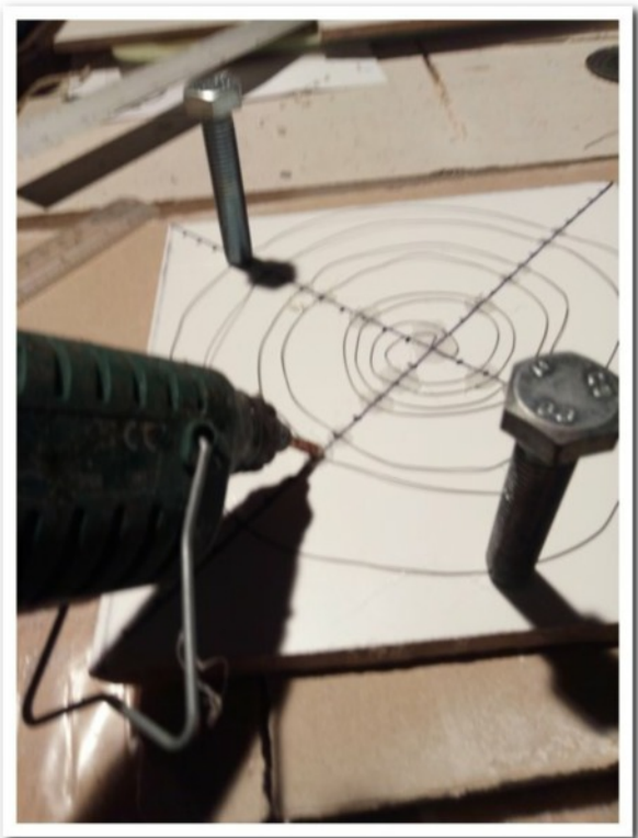
#2 Double coil wire layout - Bolts and glue gun
