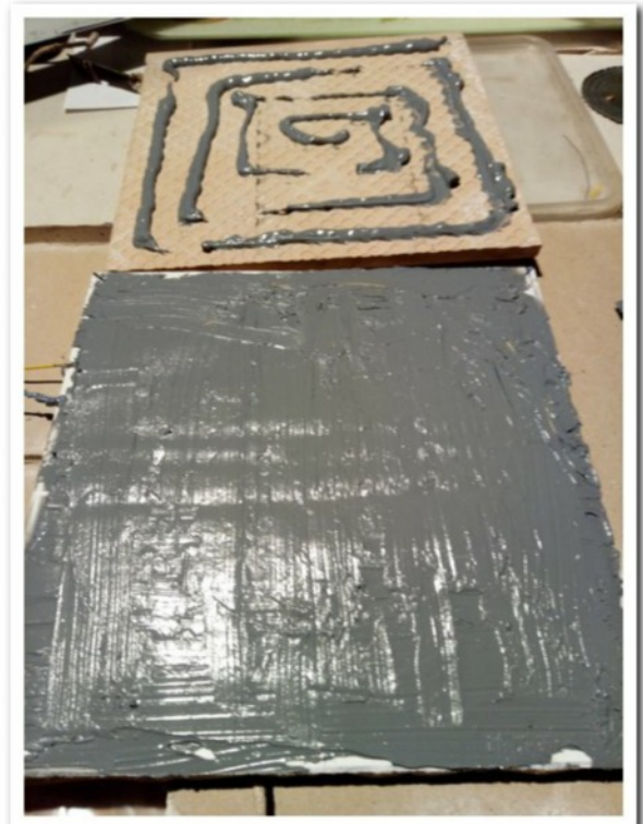
#8 Fabrication - Apply fire cement to second tile and apply to the first tile
