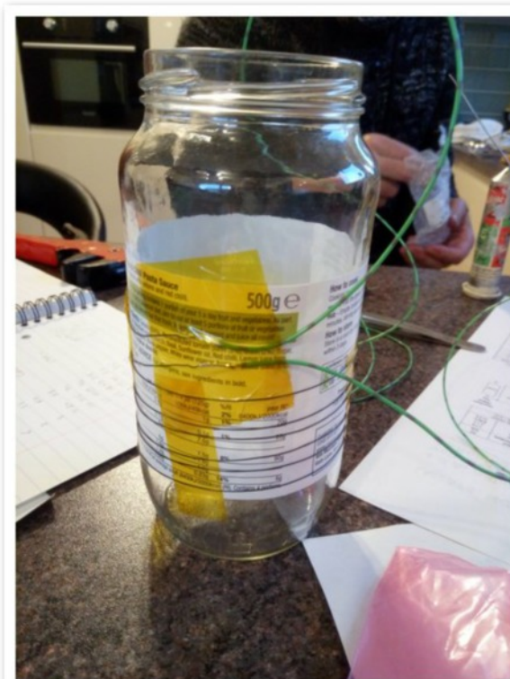
#3 Heat resistant tape being used to hold wires
