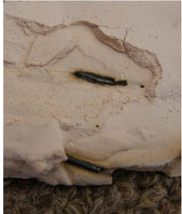
#2 Close-up of damaged heater wire
