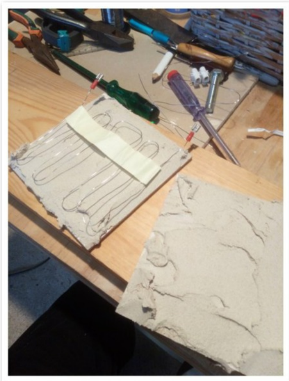
#19 Heating wire being held together using masking tape
