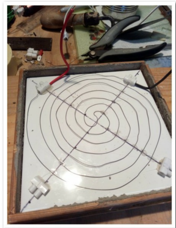
#18 Wooden frame used to hold cement and experimentation with choc block connectors
