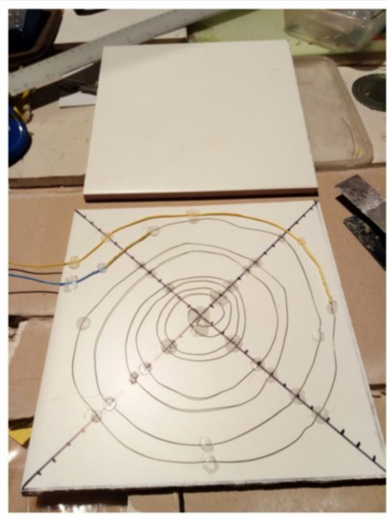
#5 Fabrication - Lay down the heat wire
