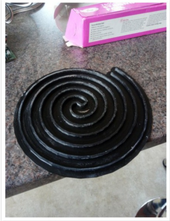
3D printed template for heater wire in clay heater plate
