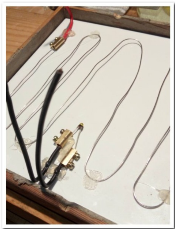
#29 Stripped choc block shown as internal connection to power/sensor wire
