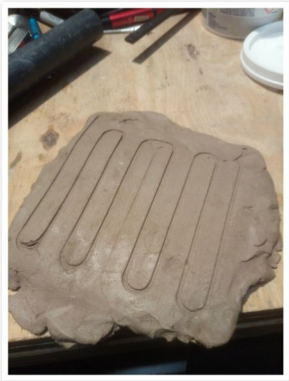
#13 Use of 3D printed profile to mark wire path in a clay
