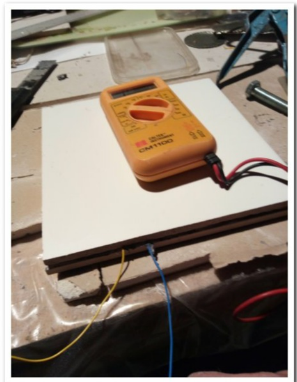
#12 After fabrication always test the wires
