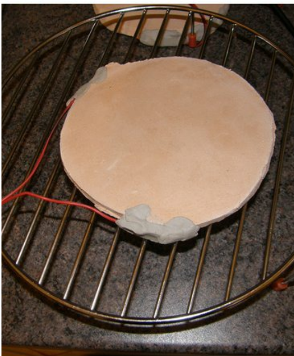
#3 Version of clay tile under heating load. Infra red photos of this tile below.
