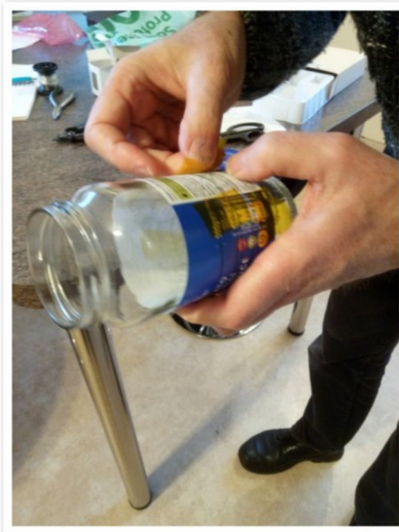
#1 Heater wire being wound onto jar
