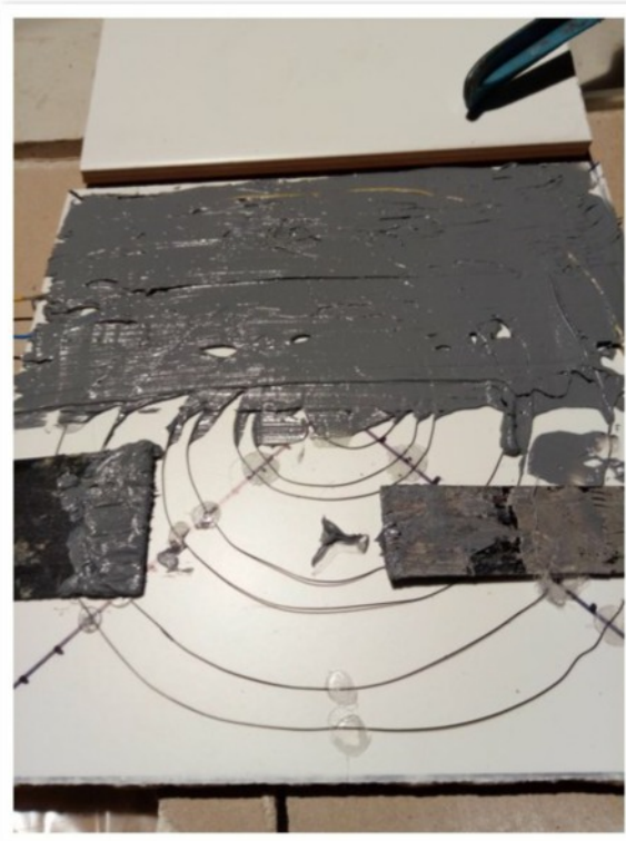
#7 Fabrication - Spread fire cement avoiding
