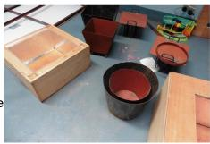
3.43 At the time of the visit it was the rainy season in Malawi and most days were overcast with little or no sun. The prototype was assembled and the functionality of the components tested. The temperature of the oil bath reached 73°C but the weather conditions prevented any further temperature rise.
