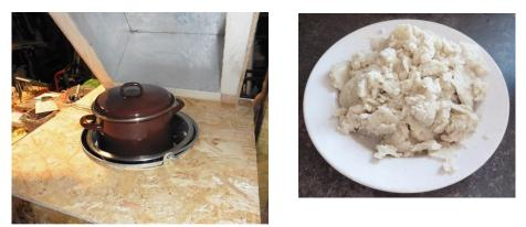
3.41 We were able to do a heating trial using a clay heater plate connected directly to a solar panel. The trial took place outside on a cold but sunny February afternoon. We were able to heat up water from 4°C to 60°C in 50 mins. At that point the sun went in and we were unable to continue the trial.
