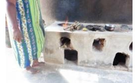
Rocket stoves are also proving popular. These stoves are available in a variety of shapes and sizes but they all have an L-shaped combustion chamber that is insulated. This chamber improves the combustion of the wood and channels the hot gases up to the cooking pot.<sup>4</sup> These means that they are more efficient in cooking the food and use significantly less fuel. Tests have shown that it uses 60% less wood fuel to boil 1L of water and simmer it for 30min.<sup>5</sup>
