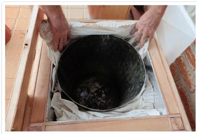
#6 Hotplate support being placed onto the base frame. One of the issues to cause concern is the seal between the base and the hotplate support. In this instance a fabric was used to close the gap
