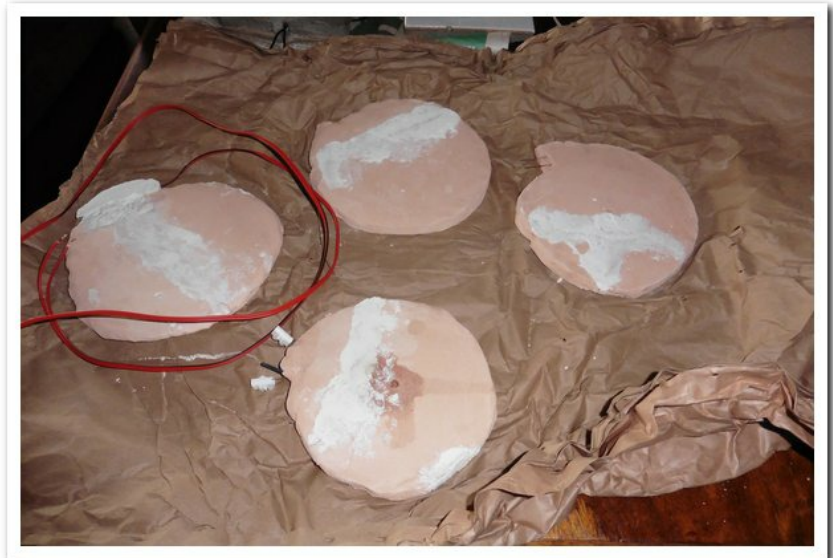
#2 Ceramic tile heaters brought from the UK. A coil of resistive heater wire also shown
