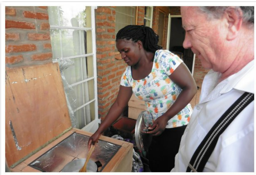
#18 The eCook stove achieved a thickened paste resembling Nsima. However there were taste differences reported by Eviness and others. The most probable explanation is that the mix was not heated to a high enough temperature
