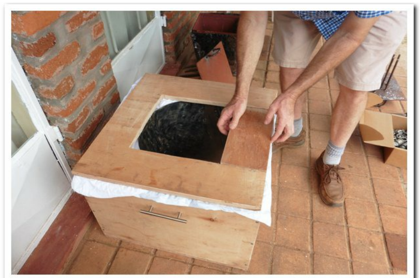
#6 Hotplate support being placed onto the base frame. One of the issues to cause concern is the seal between the base and the hotplate support. In this instance a fabric was used to close the gap
