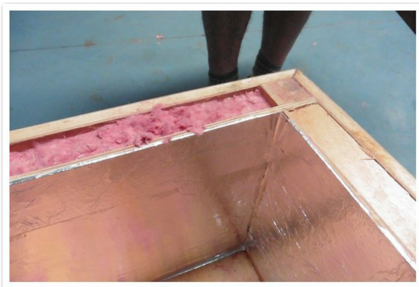
#8 Flock fiberglass insulation obtained in Malawi and fitted between the double walls of the base unit
