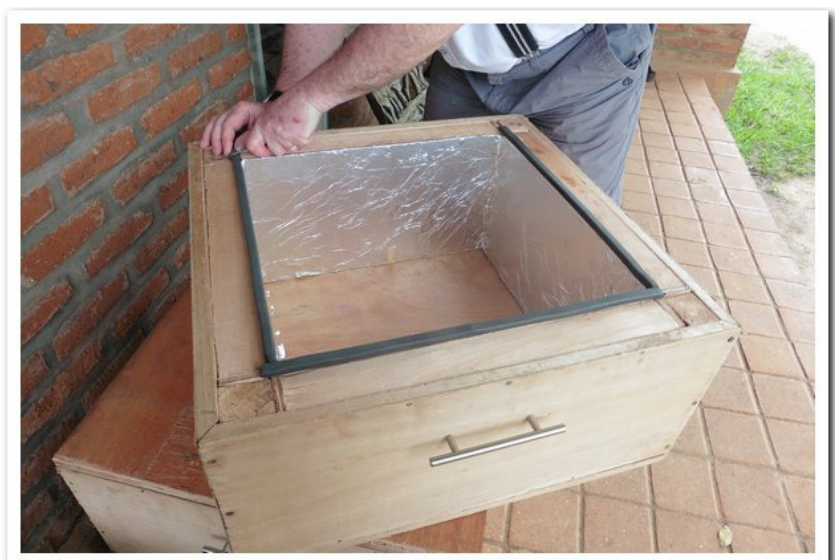
#12 Foam sealant being applied to the inside edge. This approach stopped the air path out from the vessel, but this issue needs further attention
