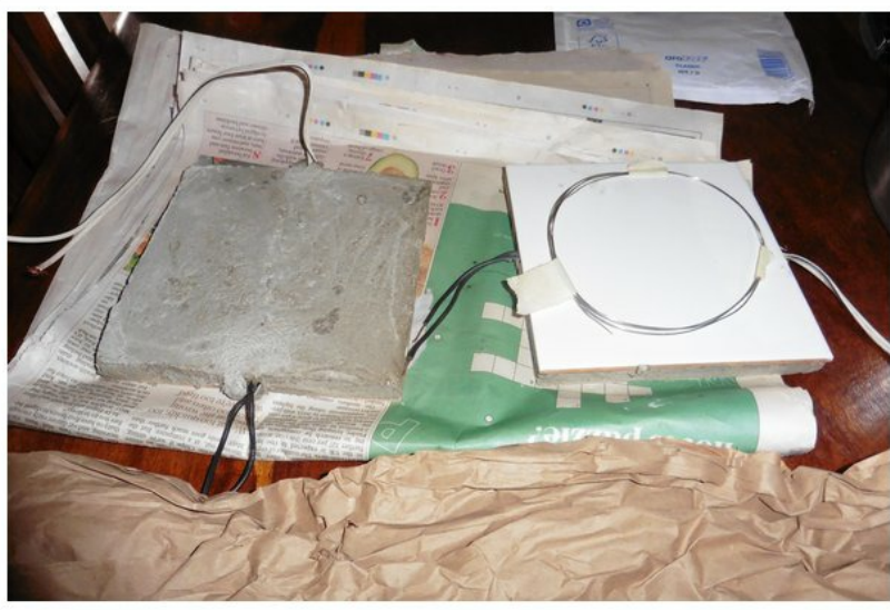
#2 Ceramic tile heaters brought from the UK. A coil of resistive heater wire also shown
